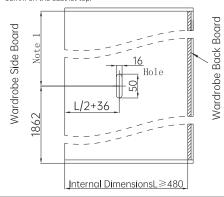
2.Please follow the instructions in the diagram and the wardrobe factory should open the wire duct in advance according to the following diagram.
