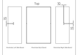
3.Set pre-embedded holes on the inner side of the side panel, or align the installation position according to the punched card.
