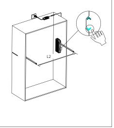
Adjust the rod distance to balance it according to the L2, ensuring that the outer cover of the pull arm matches the L2.
