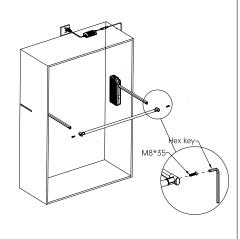
Use screws to secure the remote control holder to the appropriate position on the inside of the cabinet for storage
