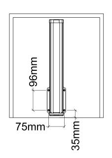
(3) fix slides onto the upper board
